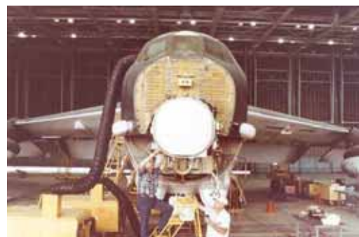
Figure 2.2-1. Electronically Agile Radar (EAR) High Energy Laser Radar Aided Targeting System (HELRATS)
