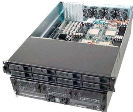
Figure 16. Quad Dual Core server computer used for passive signal beamforming and detection processing
