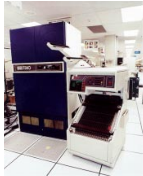
After irradiation, the LTX MTS-77 tests analog devices such as op amps and voltage regulators using software programs developed at Northrop Grumman.
